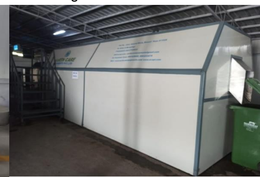
Step -7 Wet Waste + Garden Waste In Organic Waste Converter
